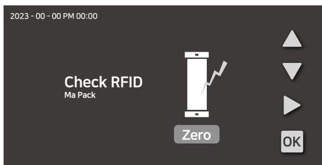
You have connected a filter that has already been used or there is an error in the reader. Contact the place of purchase or the manufacturer.
